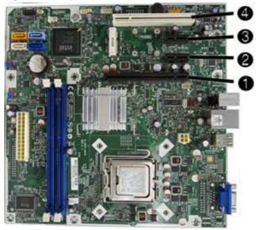
Figure 2-10 Expansion Slot Locations — 500B/510B
